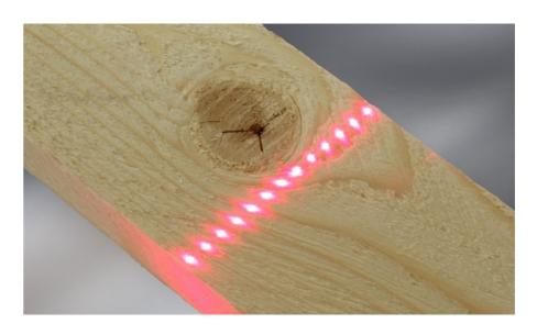
An important part of maximizing yield and profit is locating the correct cut position, especially for fingerjoint products. The scatter technology, consisting of one dot laser provides this accurracy. The dot laser will improve defect detection, especially on rough surfaces. Cut positions can be improved based on angle and shape of the dots. This helps to prevent damage in fingerjoint applications and to identify weak areas in strength grading products. Both hard and softwood can be processed.
