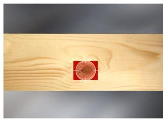
Step 3. The optimization from the powerful OptiCore software provides the best solution for cross-cutting, ripping\* or sorting. It takes into account various customer requirements and quality demands. Based on the exact characteristics identified during image processing, the board is optimized
